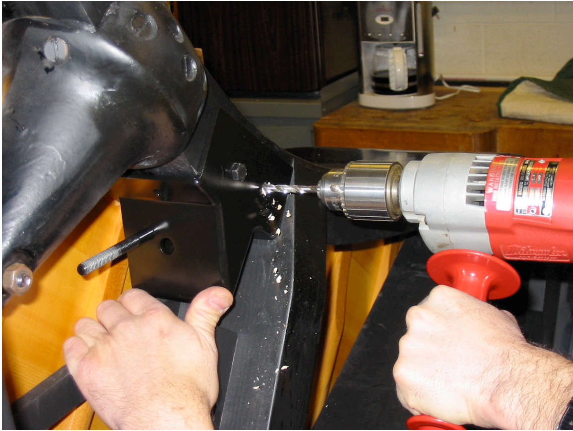
Photo 4 Weldment situated in the S-Curve for ease of drilling
