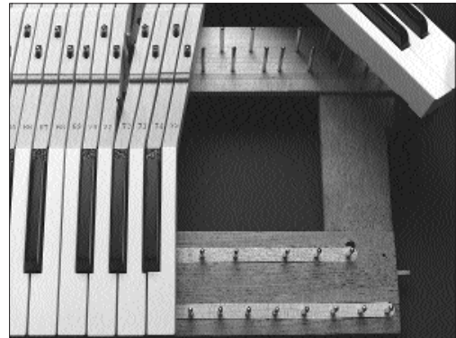
New balance rail. Front rail inlay.
